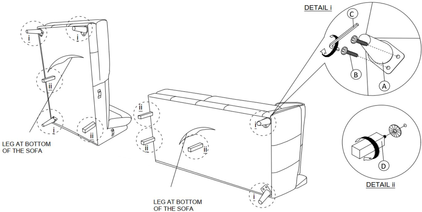
**Step 2** - To connect the lounges lift the end of piece 1 where the brackets are located and slide down onto those located on piece 2. Make sure they click firmly into place.
